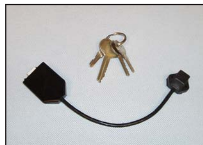
Helmet Sensor and complete tracker electronics dongle
