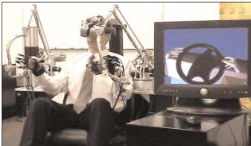
Figure 2: Haptic Workstation running the "Digital Seating Buck" application.
