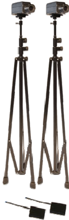
PPT H system, showing two optical sensor tracker with two infrared markers
